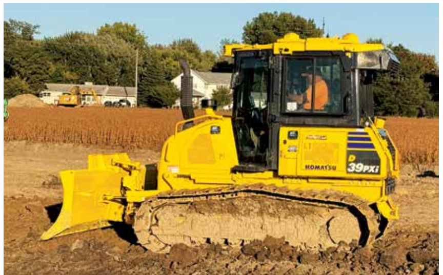
American Excavating's most recent acquisition is a Komatsu D39PXi intelligent machine control (IMC) dozer.
