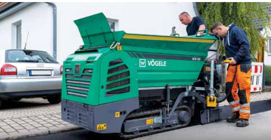
VÖGELE's MINI 500 is its smallest paver. With widths ranging from 10 inches to 5 feet, 11 inches, it is ideal for small-scale paving on limited-space sites.
