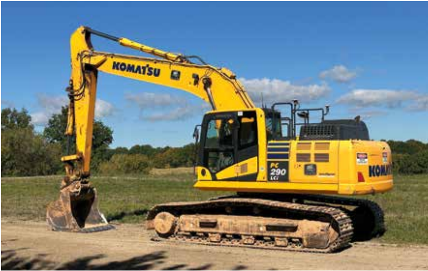
DeSal Excavating's fleet includes a Komatsu PC290LCi-11 IMC excavator.
