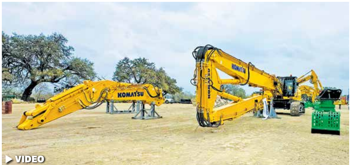
Komatsu's new PC490HRD-11 high-reach demolition excavator features a K100 boom change system for faster reconfigurations.
