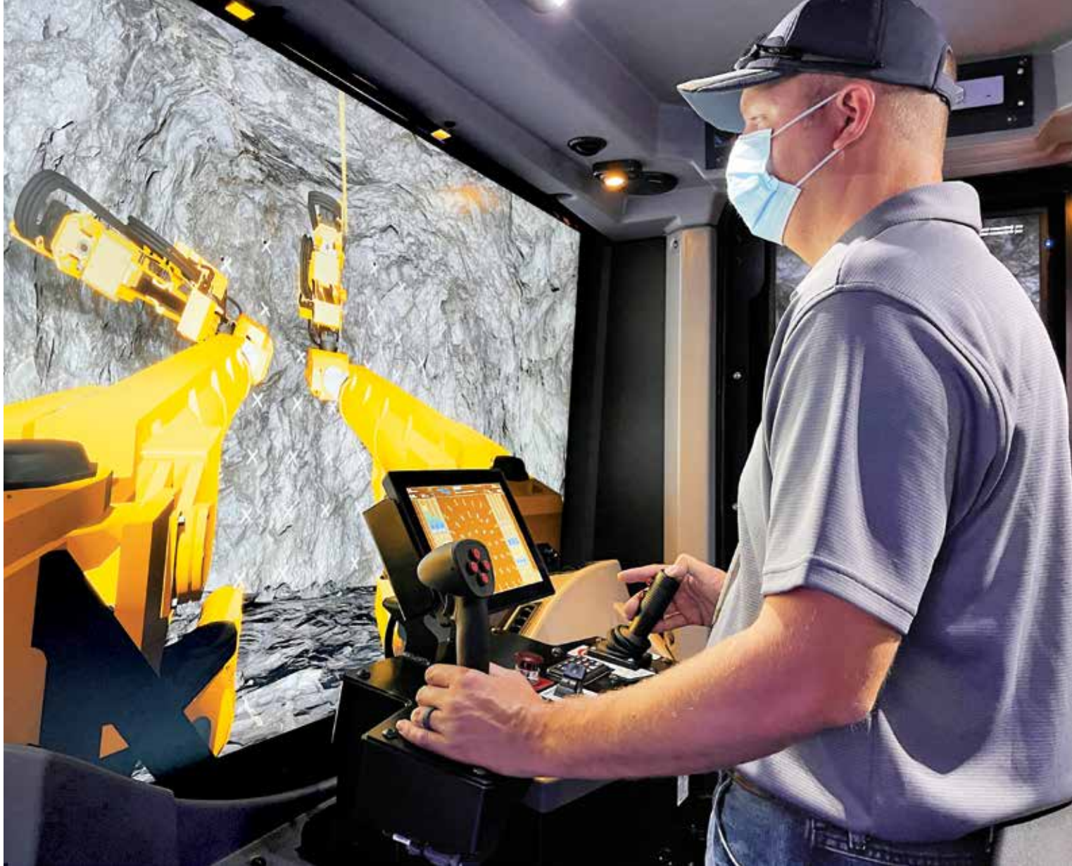
Simulators can help trainees understand how to operate machinery before they get in the actual cab and may also be a way to prepare for remote machine operation.
