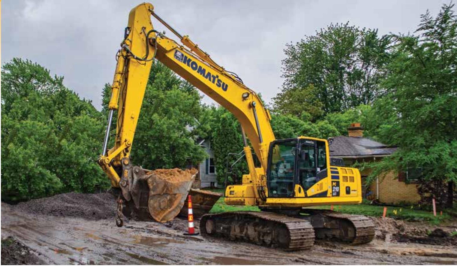
Tri-City Groundbreakers Owner John Schmidt uses a Komatsu PC210LCi-11 excavator with intelligent Machine Control at the Trumbull Street project in Bay City, Mich. “We purchased the PC210LCi this spring, and the results have been great,” shared John. “Having the ability to dig on grade is amazing, and we don’t need a person in the hole, which increases our efficiency.”
