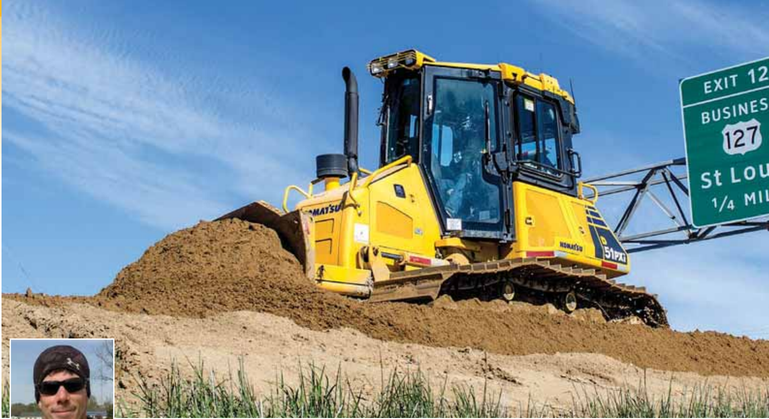
Foreman Reggie Smith uses one of Malley Construction's Komatsu intelligent Machine Control D51PXi dozers to grade a shoulder. "Everything works together so well on the D51PXi, it's amazing," said Smith. "I was blown away by the speed at which I can finish grade. It actually runs better at max speed. It carries better, the grade is smooth and you finish faster."
